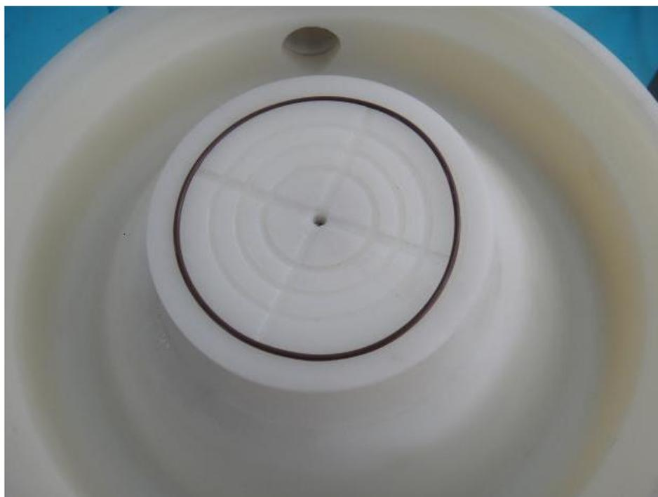
4. Visually inspect the spinning head which drives the vacuum chuck and clean it by using pure ethanol if there are any residues.
